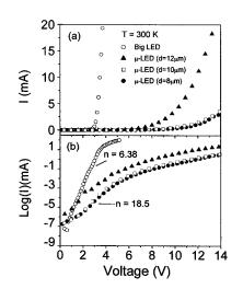
FIG. 2. I-V characteristics of  $\mu$ -LEDs of varying sizes (d=8, 10, and 12  $\mu$ m) and a broad-area LED ( $300 \times 300 \ \mu$ m<sup>2</sup>) in (a) linear and (b) semilogarithmic plots.
