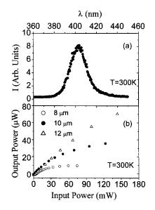
FIG. 3. (a) EL emission spectrum of a purple  $\mu$ -LED. (b) Output power vs input power (L-I) plot of  $\mu$ -LEDs of different sizes.
