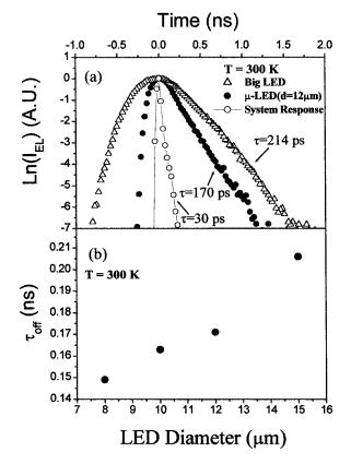
FIG. 4. (a) Transient response of a  $\mu$ -LED and a conventional broad-area LED. (b) Size dependence of the turn-off time,  $\tau_{off}$ , of  $\mu$ -LEDs.
